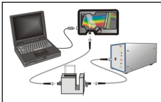
Absorbance is also proportional to the concentration of the substance interacting with the light (this is known as Beer's Law). Common absorption applications include the quantification of chemical concentrations in aqueous or gaseous samples.
