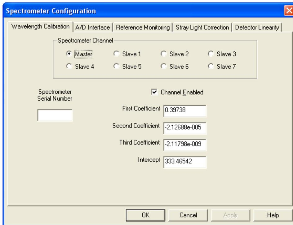
2. The **Wavelength Calibration** tab is selected. OOIBase32 should automatically load the coefficients for each spectrometer channel in your system from the .SPEC file you specified. If OOIBase32 did not load these values, manually enter the calibration values provided on the Wavelength Calibration Data Sheet that came with your spectrometer.
