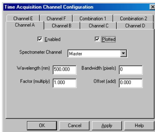
The following options are available from the Channel tabs on the Time Acquisition Channel Configuration dialog box.
