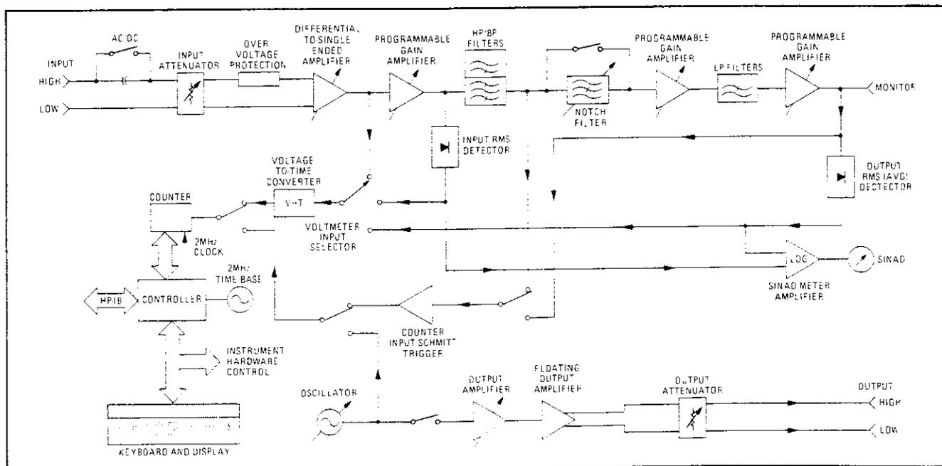
Figure 1-5. Simplified HP 8903A Audio Analyzer Block Diagram
