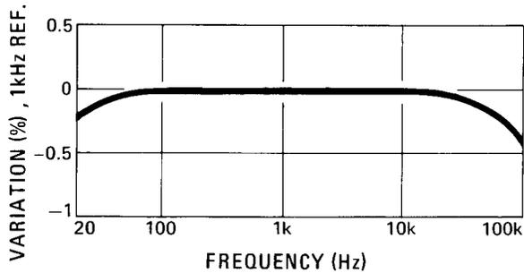
Figure 1-2. Typical Combined Source and AC Level Flatness
