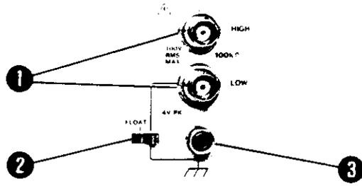
**1 INPUT HIGH and LOW Connectors.** Used to connect the device under test to the analyzer. When the FLOAT switch is in the FLOAT position, both connectors are used. If the switch is in the grounded position a single BNC-connector can be connected to the HIGH input. Input impedance is 100 kΩ (101 kΩ, dc level only).
