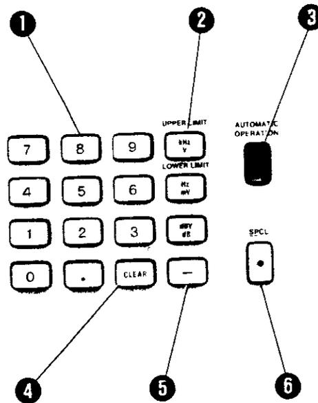
**1 Numeric Keys.** Used to enter source frequency and amplitude, incremental values, ratio references, sweep start and stop frequencies, plot limits, and to select Special Functions. Numeric entries are completed by the **RATIO**, **kHz/V** (**UPPER LIMIT**), **Hz/mV** (**LOWER LIMIT**), **dBV/dB**, or **SPCL** keys. Numeric entries in progress are cleared by the **CLEAR** key.
