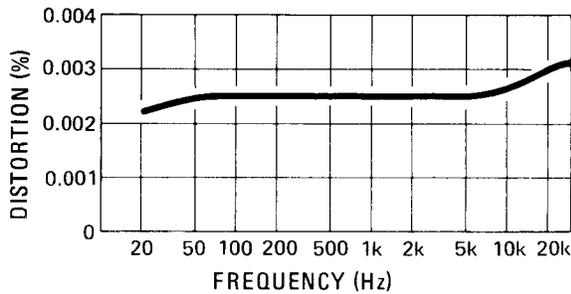
Figure 1-3. Typical Combined Source and Analyzer Residual Distortion
