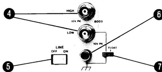
**4 OUTPUT HIGH and LOW Connectors.** Used to connect the source to the device under test. When the FLOAT switch is in the FLOAT position, both connectors are used. If the switch is in the grounded position, a single BNC-connector can be connected to the HIGH output. Output at the connectors is 0.60 mV to 6V (open circuit), 20 Hz to 100 kHz, with 600 Ω impedance.
