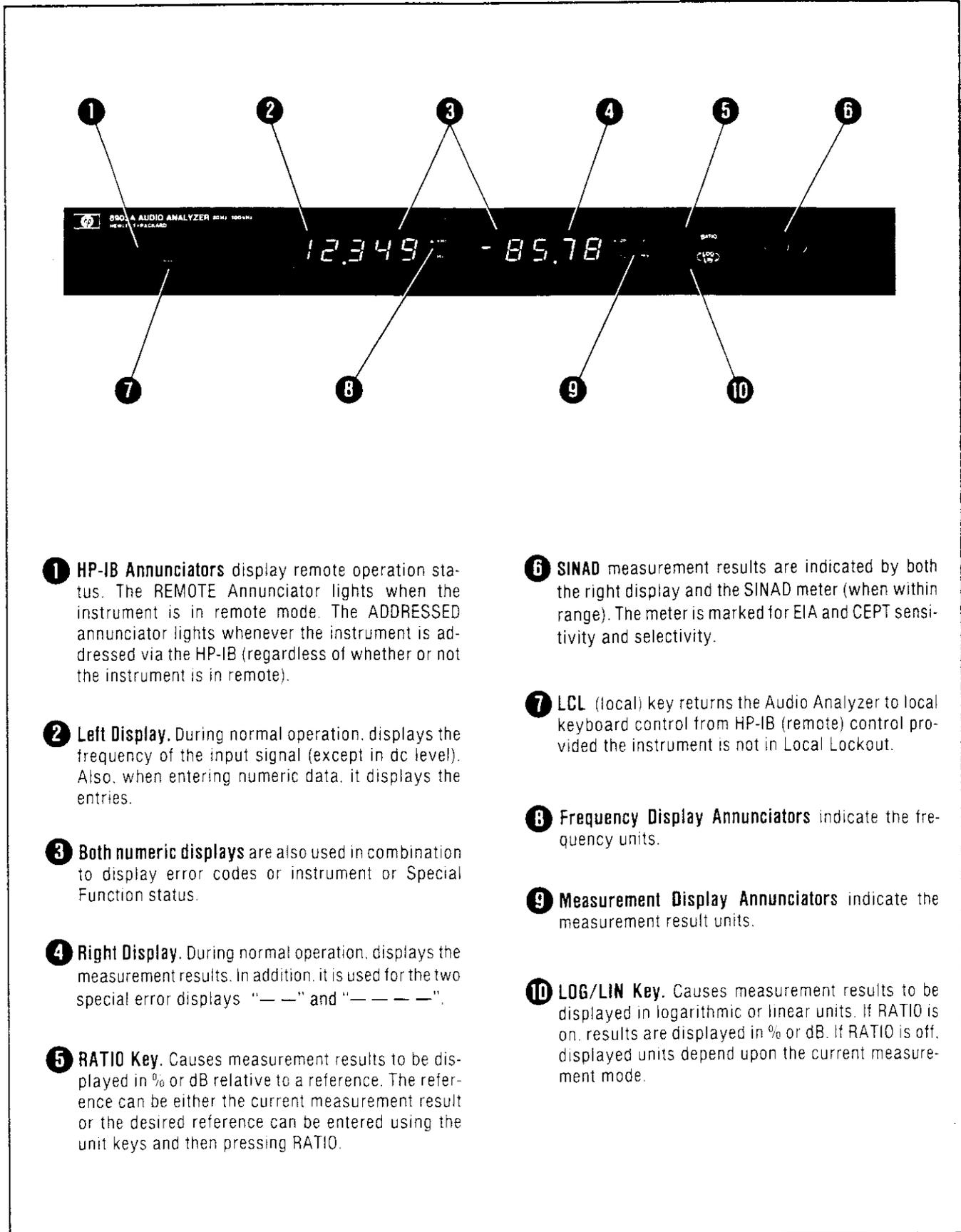
**1 HP-IB Annunciators** display remote operation status. The REMOTE Annunciator lights when the instrument is in remote mode. The ADDRESSED annunciator lights whenever the instrument is addressed via the HP-IB (regardless of whether or not the instrument is in remote).
