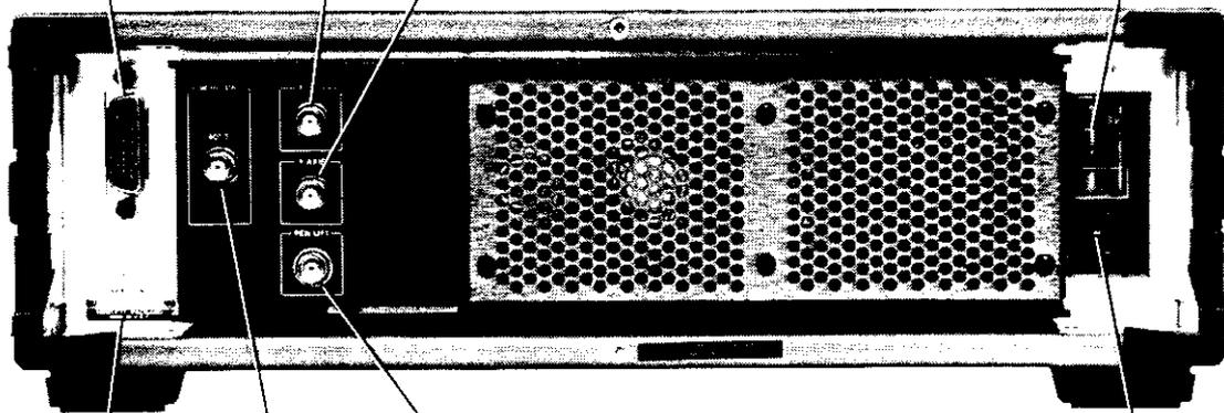
**Line Power Module** permits operation from 100, 120, 220, or 240 Vac. The number visible in window indicates nominal line voltage to which instrument must be connected (see Figure 2-1). Center conductor is safety earth ground.
