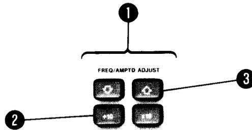
**1 FREQ/AMPTD ADJUST Keys.** These keys are used to manually adjust the frequency and amplitude of the source.
