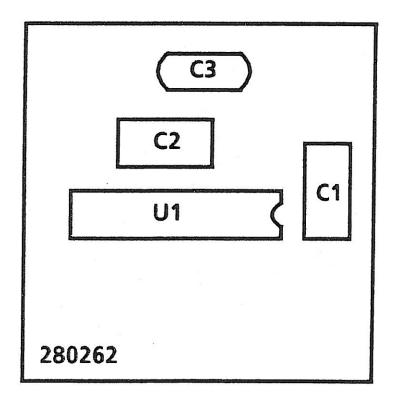
Figure Q-1. Part 280262-1, Keyboard Encoder (Option Q - PKC), Location of Components
