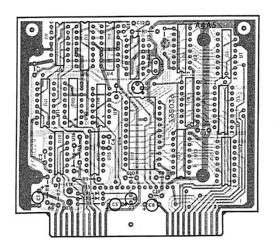
Figure O-1. Type 798029-1, Variable BFO (A4A5) (Option O - VBFO), Location of Components
