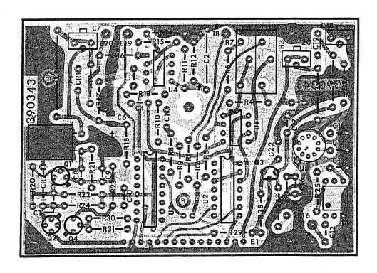
Figure O-2. Part 390343-1, Oscillators (A4A5A1), Location of Components
