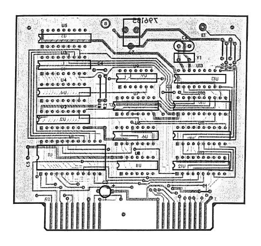
Figure M-1. Type 796185-6 Real Time Clock, (Option M-RTC) Location of Components
