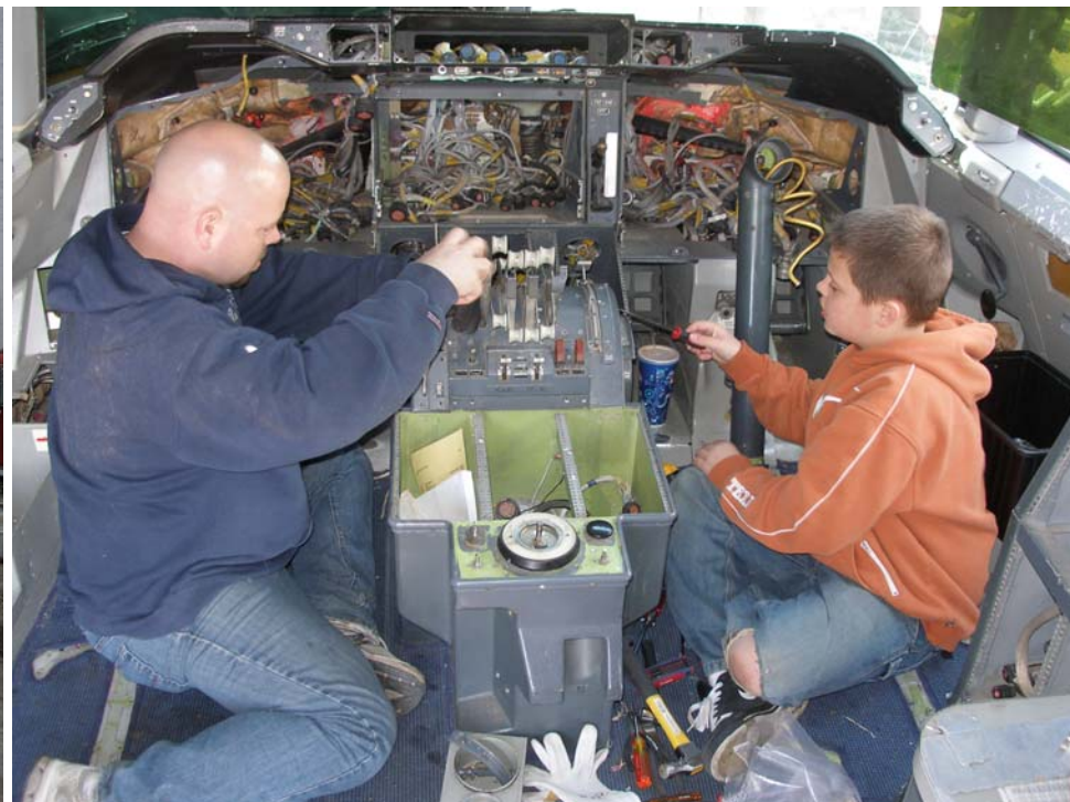
As the cockpit was to be stored at the wrecker's yard for several weeks, all control panels, flight controls, seats, carpet and interior Trim was removed to ensure nothing was left that could be stolen
