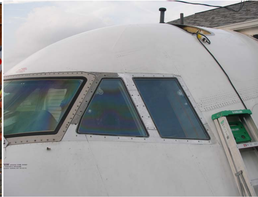
Very little restoration was required on the exterior before painting except the polishing the grime off of the aluminum side window frames
