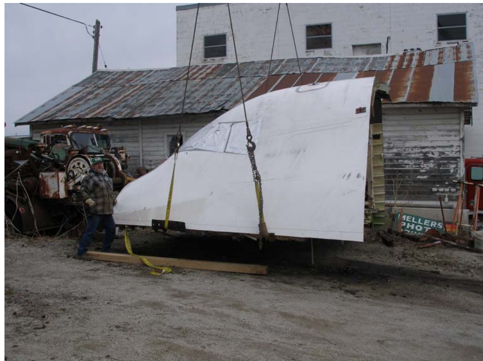
The cockpit was lowered onto wood planks to avoid the sharp Cut edges from digging into the ground and making difficult to Place straps beneath it for its final delivery to the house
