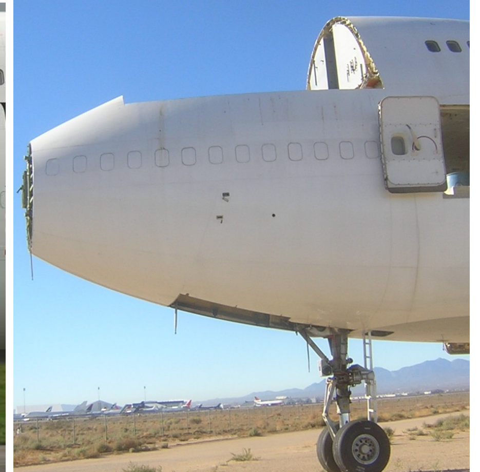
Same aircraft with the cockpit removed. Was cut further forward than necessary for easy removal, then trimmed further on ground
