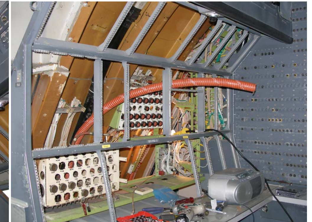
The Flight Engineer's station was especially time-consuming to de-wire
